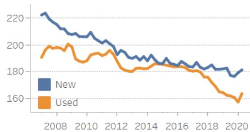
Figure 4d: Average tailpipe CO<sub>2</sub>/km of light registrations by fuel (including PHEVs)
